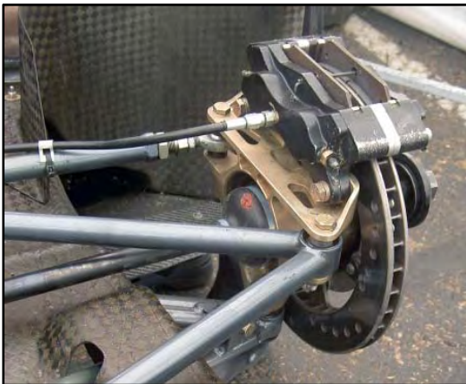
Rear Suspension Upright as Installed on J.R. Osborne's Stohr DSR
