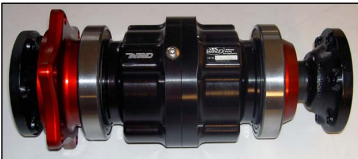
Luxon Engineering Designed WRD Differential
